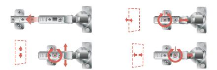
• You can turn the push-to-open pin. This closes the door further inwards or outwards. You can also try this when the push-to-open system does not work properly. The pin is then given more or less space to push in and push out properly.
